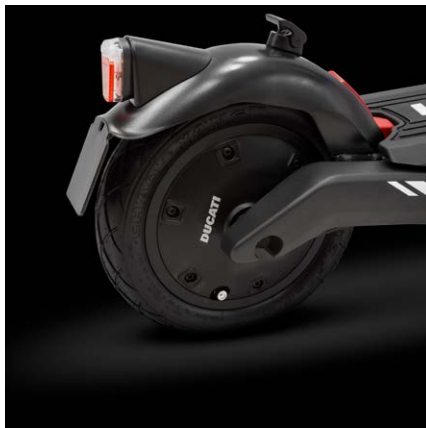
Motore 500W, Peak Power: 800W
